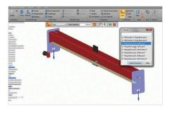
Once everything is set up, you can mesh and solve the study. Solid Edge gives users complete control over the mesh settings for both solid and surface meshes. You can easily change your view of results; for example, from stress distribution to displacement using a dropdown.
